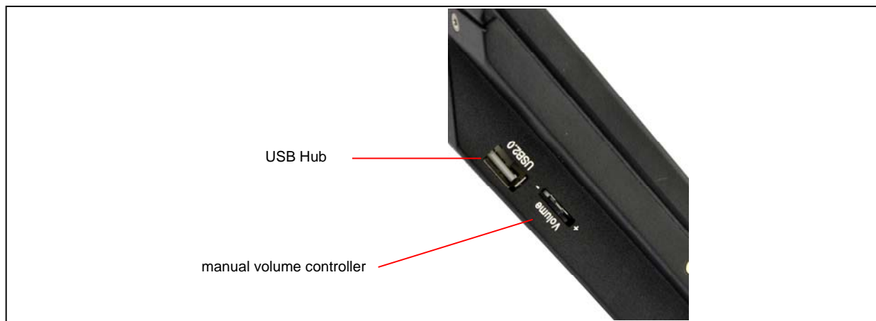
Figure 6: Manual volume control on the left side of the monitor (DMXX1132)
